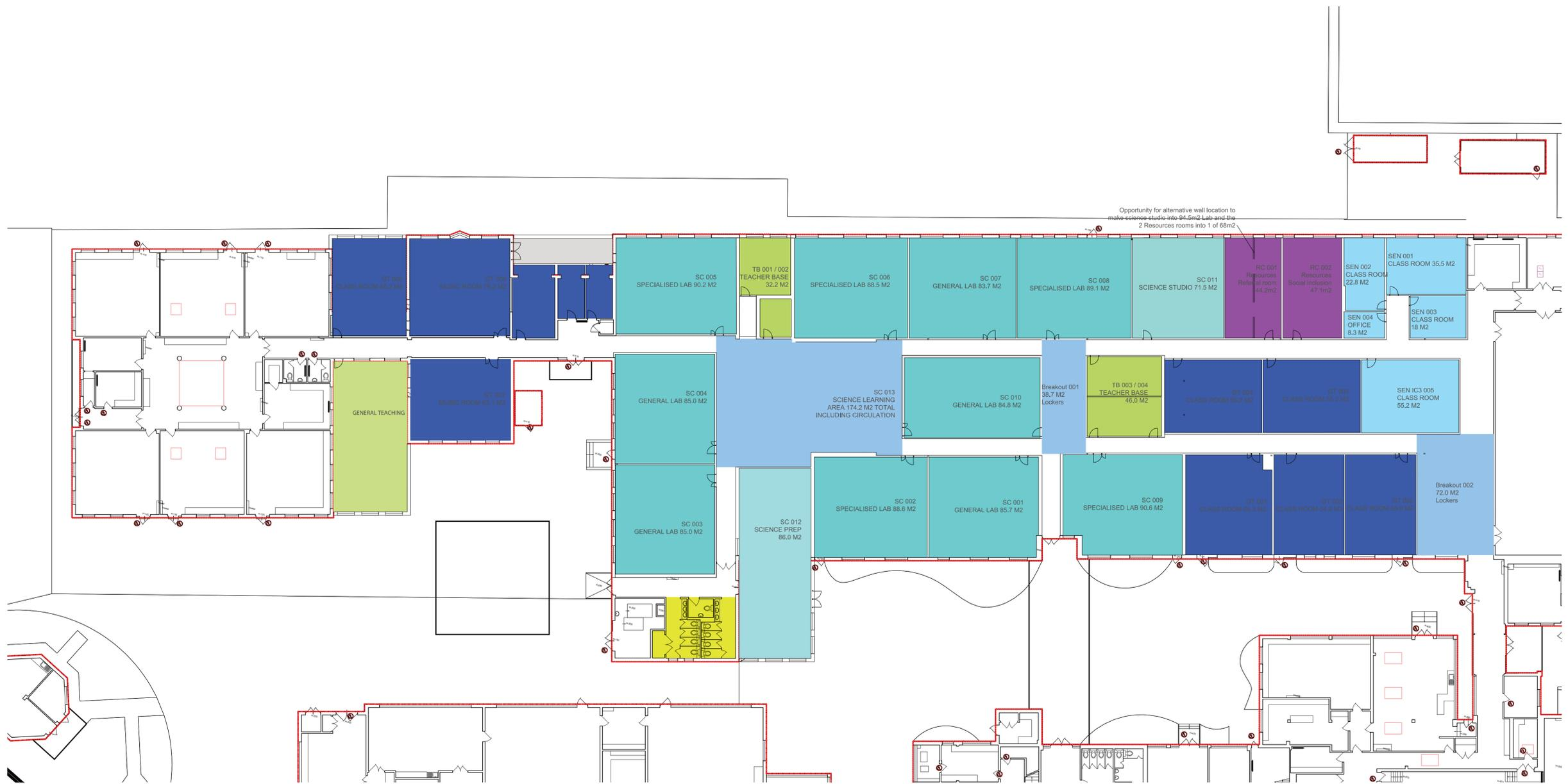
Reconfigure existing layout. New roof structure to central area to allow for openable windows for improved lighting and ventilation. Refurbish existing toilet block. Retain as much of the existing exterior classrooms and layout as possible and mainly reconfigure central core.
